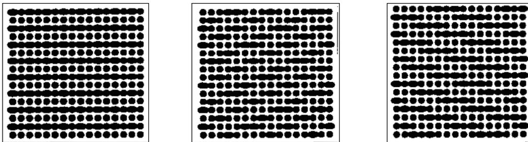
Figure 3. Breaking the horizontal bands produced by elliptic dot shapes with distributions of dither thresholds according to the tiles shown in Fig. 2a and 2b.
