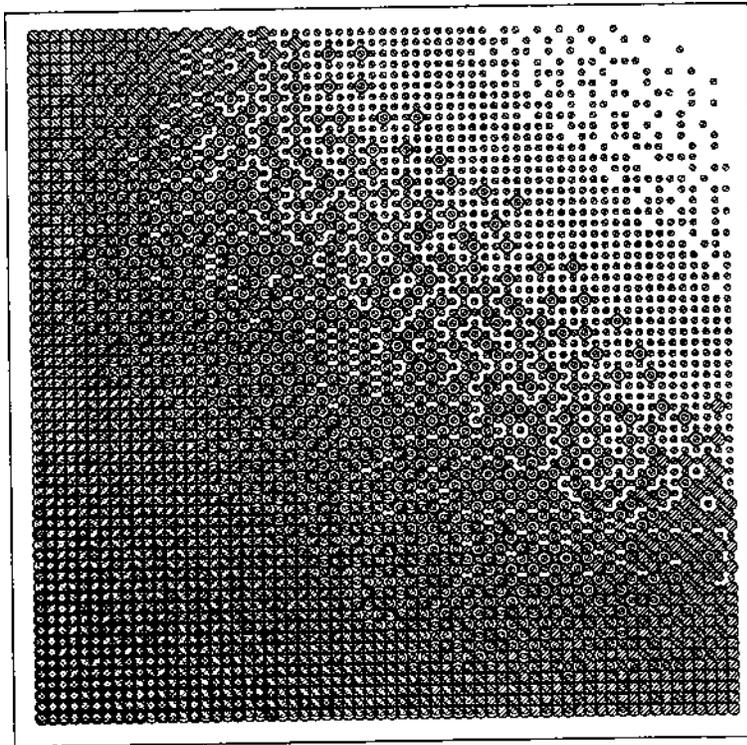
Figure 8. Variable dot size colour error-diffused cyan magenta wedge, with intensity-dependent inhibiting constraints (blue 50% discarded).
