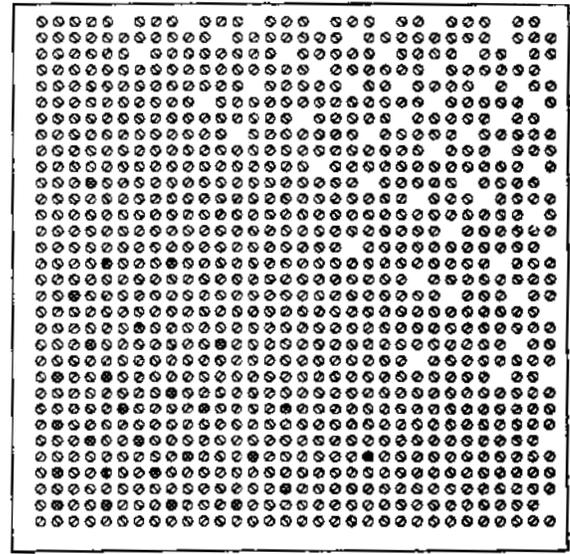
Figure 5. Bilevel colour error-diffused patch with surface coverages  $c_1 = 50\%$ ,  $c_2 = 50\%$  at the center and with  $\pm 12\%$  coverage increase/decrease towards the edges
