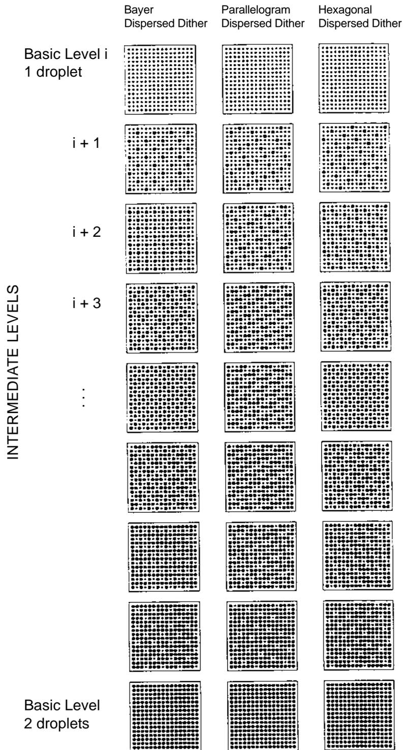
Figure 9. Intermediate intensity levels produced by dither tile based multi-level printing; The parallelogram dither corresponds to the tile shown in Fig. 2a and the hexagonal dither to the tile shown in Fig. 2b.
