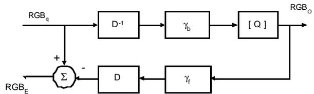
Figure 3. Color correction model for the devices with limited output colors.
