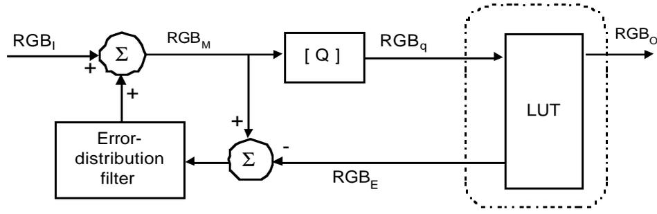
Figure 6. Equivalent combined model of error diffusion and color correction.
