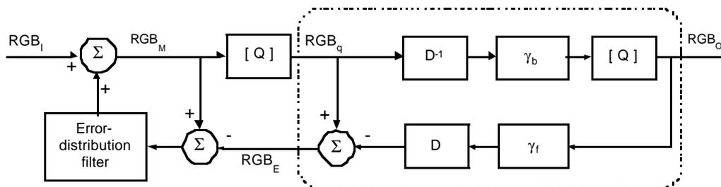
Figure 5. Combined model of error diffusion and color correction.
