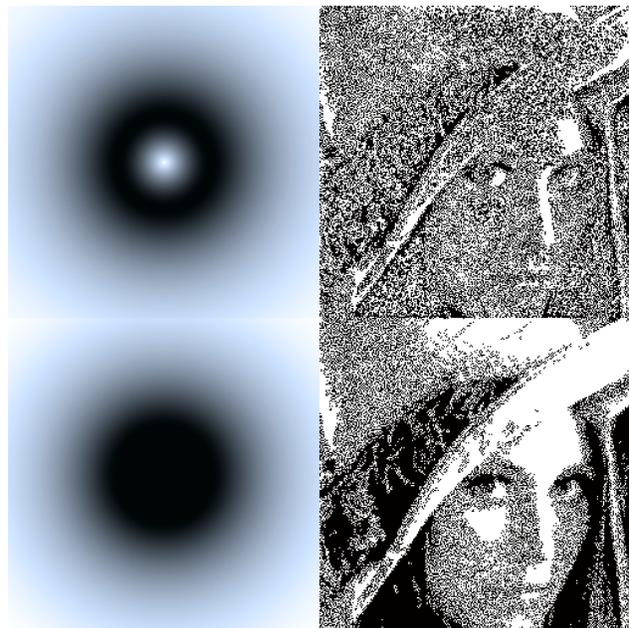
Figure 1. From left to right and top to bottom: (a) inverted CSF filter (b) halftone output using inverted CSF filter (c) inverted low-pass modified CSF filter (d) halftone output using inverted low-pass modified CSF filter.
