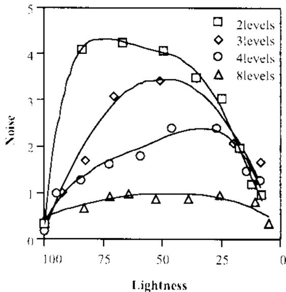
Figure 2. Effect of number of quantization levels on dot noise.
