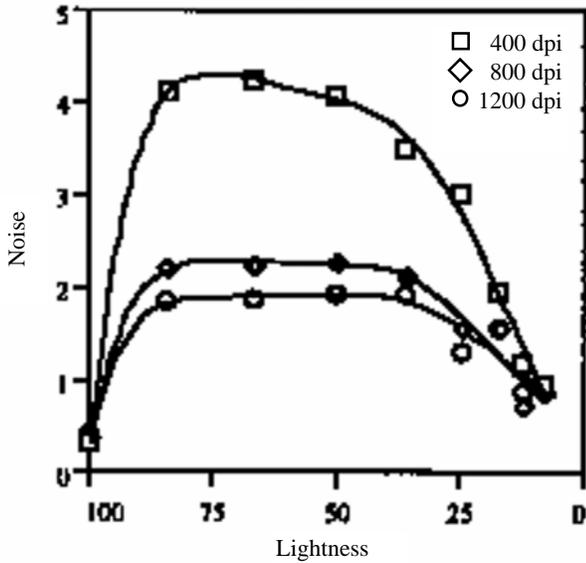
Figure 3. Effect of resolution on dot noise
