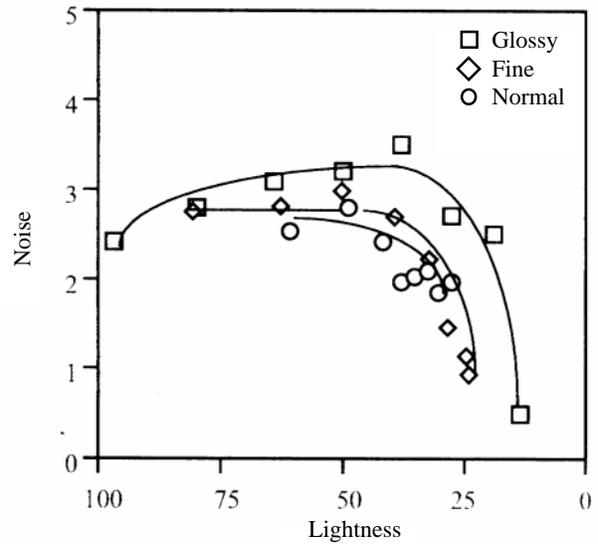
Figure 4. Effect of paper substrate type on dot noise
