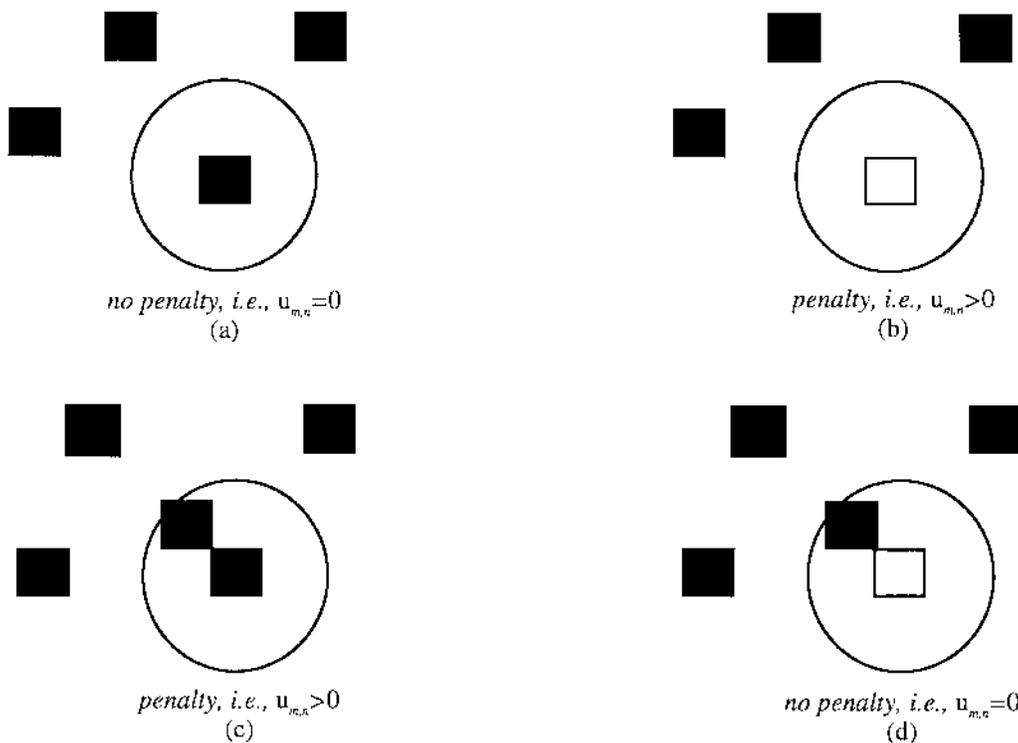
Figure 3. Examples showing the four different situations in the dot distance based distortion measure of (6). In these examples, we have  $g = 0.75$ ,  $r = 0$  (minority pixel is black) and  $d_p(g) = 2$ . The circle in each case is of radius 2, which equals the principal distance  $d_p(g)$  at the graylevel used in this example.
