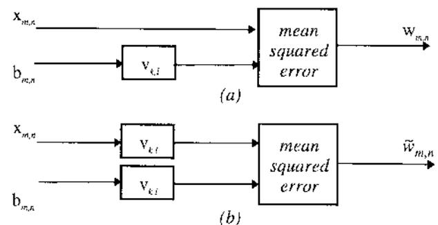
Figure 1. Two different forms of frequency weighted mean squared error.
