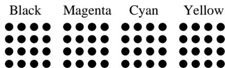
Figure 2 Print Nozzle Arrangement for Passive Fault Tolerance
