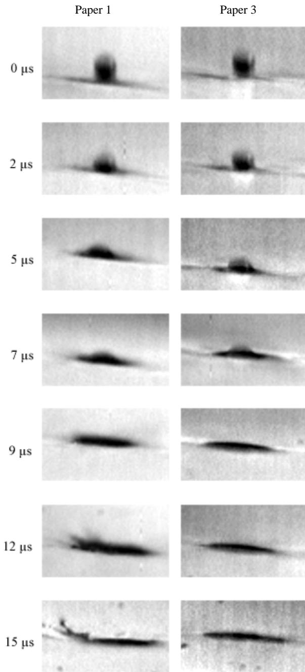
Figure 2: The behaviour of the ink drops on Papers 1 and 3 during the first fifteen microseconds after the impact. The splashing on Paper 1 began after 12  $\mu$ s. The splashes can be seen on the left-hand side of the drops, because the substrate was running at 10 m/s from the left to the right.
