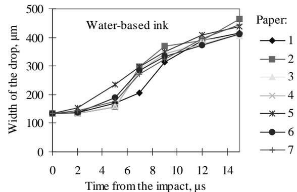
Figure 3: The spreading of the water-based ink on the paper samples. Five to seven microseconds after the impact differences were observed in the shapes of the drops on the different substrates.
