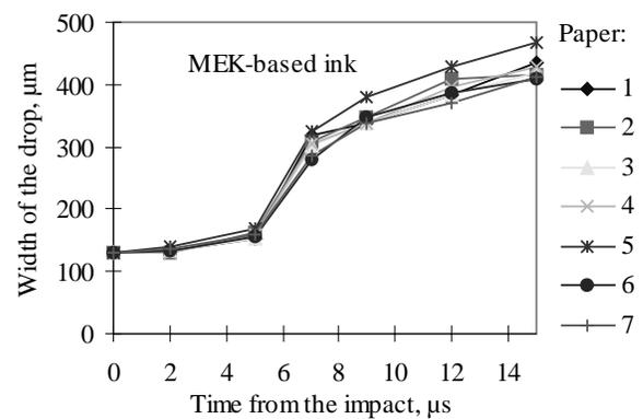
Figure 4: The spreading of the MEK-based ink on the paper samples. The MEK-based ink was found to be less sensitive to the paper properties than the water-based ink.
