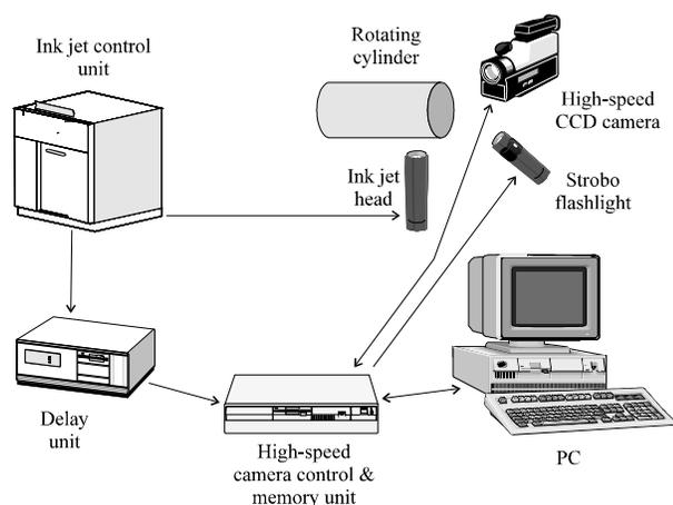
Figure 1: The experimental arrangement for the high-speed imaging of ink jet drops.
