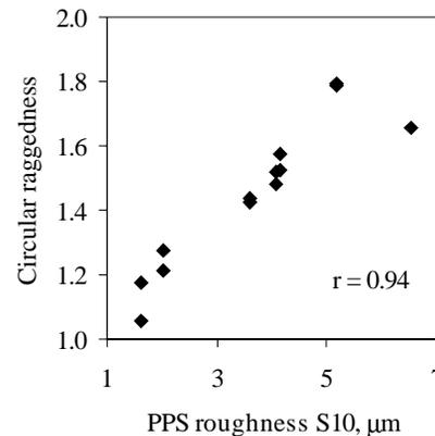
Figure 6: Circular raggedness as a function of the Parker Print Surf roughness.
