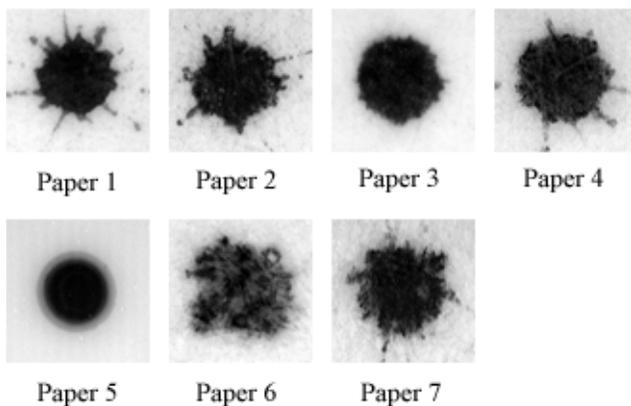
Figure 5: Examples of the dots printed with the water-based ink on the substrates. When these dots were printed, the velocity of the substrate was only 3.5 m/s and the splashes occurred anywhere around the drops.
