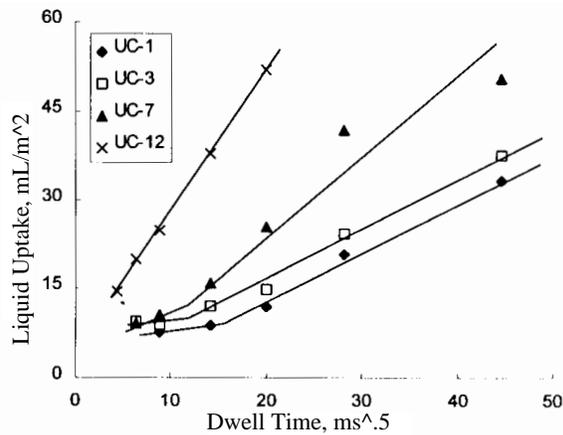
Figure 2. Bristow Absorption Tester Liquid uptake - Time curves for wetting time and absorption rate determinations.
