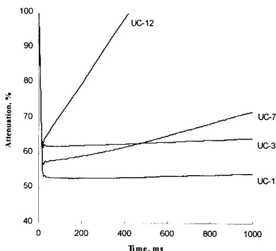
Figure 1. Ultrasonic Wettability Tester Attenuation - Time curves for wetting time and absorption rate determinations
