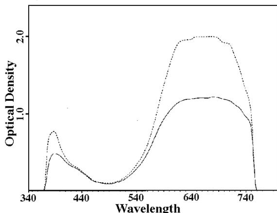
Figure 2. A comparison of the reflection spectra for the small cyan (dashed line) and the big cyan (solid line) pigmented inks.
