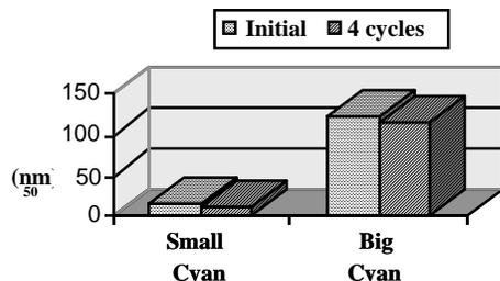
Figure 1. The effect of 4 freeze/thaw cycles on the cyan inks of this study.
