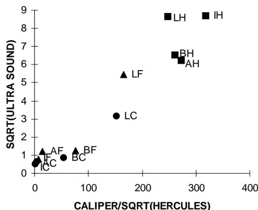
Figure 3: Correlation between the ultrasound attenuation and Hercules sizing.
