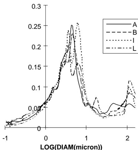
Figure 1: Derivative of the cumulative pore volume with respect to the log of the diameter vs. pore diameter by mercury porosimetry
