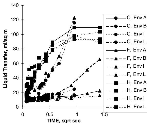
Figure 4 Liquid uptake for inks C, F and H and envelopes A, B, I and L.
