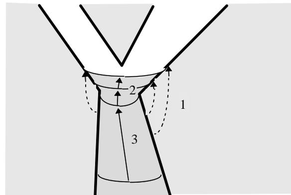
Figure 7: Ink absorbs by: (1) diffusion past pinning sites (2) and capillary jumps (3) driven by surface energy.
