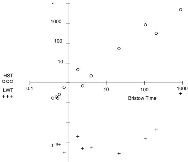
Figure 6: Comparison of LW calculated speed and experimental times obtained from Bristow and HST.
