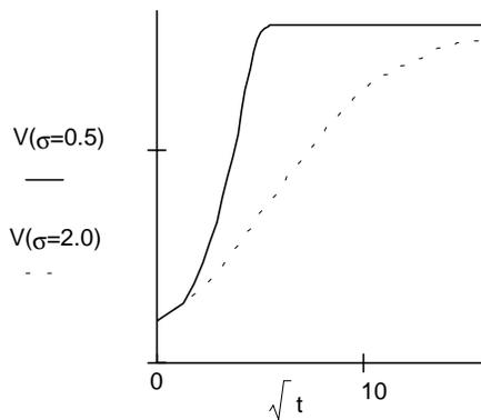
Figure 9: Monte Carlo calculation of Bristow curves from pinning model with  $\sigma$  of 0.5 and 2.0. The mean pinning time is normalized to 1.
