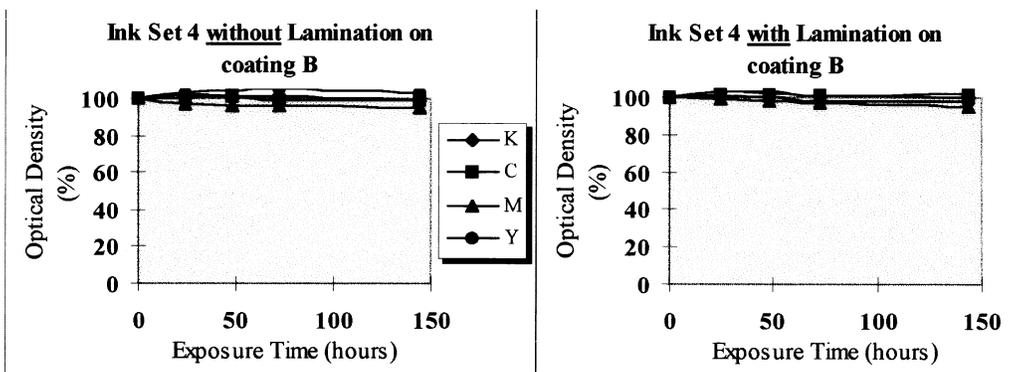
Fig. 10: Accelerated light exposure of ink jet prints with ink set 4 on coating B.
