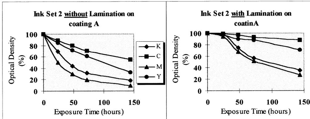
Fig. 6: Accelerated light exposure of ink jet prints with ink set 2 on coating A.
