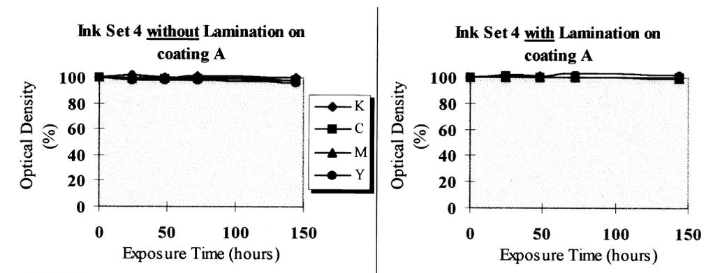
Fig. 9: Accelerated light exposure of ink jet prints with ink set 4 on coating A.
