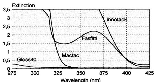
Figure 1. Spectral absorption of lamination films.
