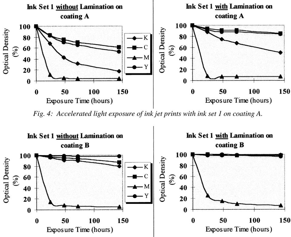
Fig. 4: Accelerated light exposure of ink jet prints with ink set 1 on coating A.
