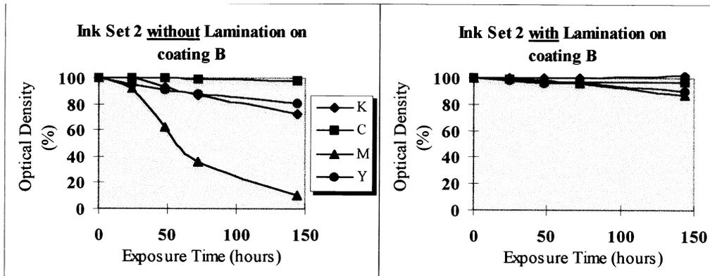
Fig. 7: Accelerated light exposure of ink jet prints with ink set 2 on coating B.
