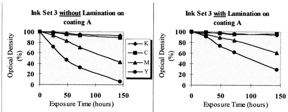
Fig. 8: Accelerated light exposure of ink jet prints with ink set 3 on coating A.
