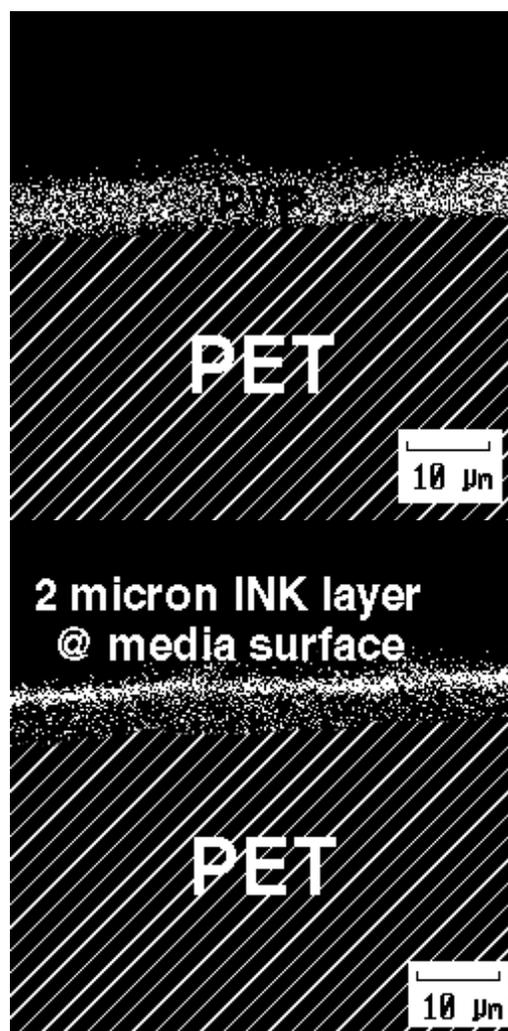
Figure 5. PVP image at 112<sup>+</sup> + 124<sup>+</sup> for inked cross-sections of HP Premium Glossy film; ink signals at 87<sup>+</sup>, 89<sup>+</sup>, and 480<sup>+</sup>-552<sup>+</sup>.
