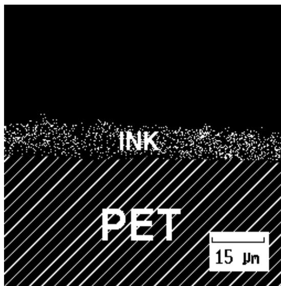
Figure 2. The negative ion mode cross-sectional image of the magenta dye-characteristic  $\text{SO}_3^-$  ion at  $80^-$  for the inked **PVOH** film.
