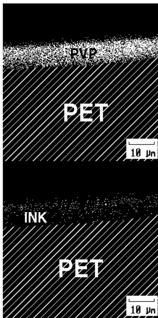
Figure 8. The negative ion mode image of the PVP-characteristic ions at 26°, 42°, and 84° in a cross-section of the Pollectron (PS/PVP) film and the sulfonate ion ( $\text{SO}_3^-$ ) image at 80° due to the ink.
