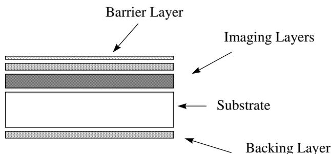
Figure 4 Structure of a barrier coated media. Such a technique can render the media virtually insensitive to the effects of humidity on print quality.
