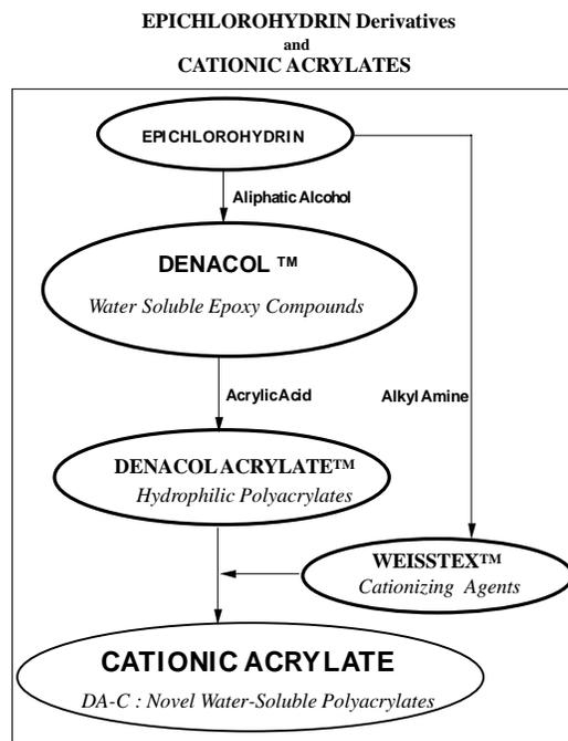
The principal synthetic root of cationic acrylate, DA-C, is shown in above diagram. The schematic formula of DA-C is as follows.
