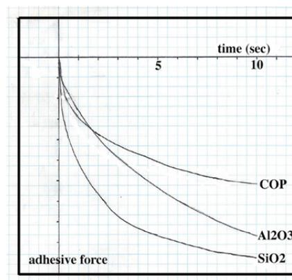
Figure 7. Wetting curve of COP with ink mean particle size of test samples; COP:300nm, Al<sub>2</sub>O<sub>3</sub>:100/10nm, SiO<sub>2</sub>:700/15nm (aggregate/primary)
