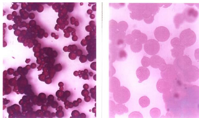
Figure 5. Swelling of spherical COP by aqueous ink; left : before swelling; right : after absorbing magenta ink
