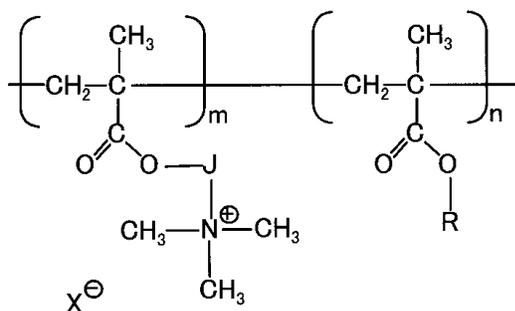
Figure 6. Cationic polymer suitable for ICOS particles
