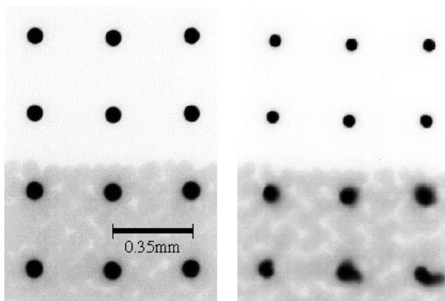
*Figure 5. Dot shapes on a microporous paper print (left) and a swelling paper print (right). In the top half, only black dots are printed, in the bottom half, black dots are printed against a field of yellow dots.*
