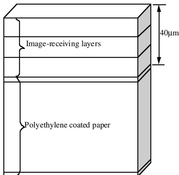
Figure 1. QP paper layer structure
