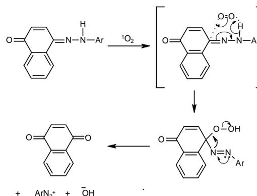
Figure 5. The oxidative destruction of an azo chromophore
