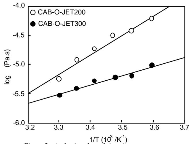
Figure 5. Arrhenius plots of viscosity for CAB-O-JET 200 and 300
