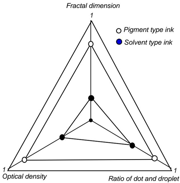
Figure 8. Evaluation triangle composed by 3 parameters for two type inks on PPC paper
