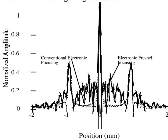
Figure 4. Simulated ultrasonic beam profiles in the azimuth plane at a focal length of 2.5 mm using electronic focusing with 16 elements.
