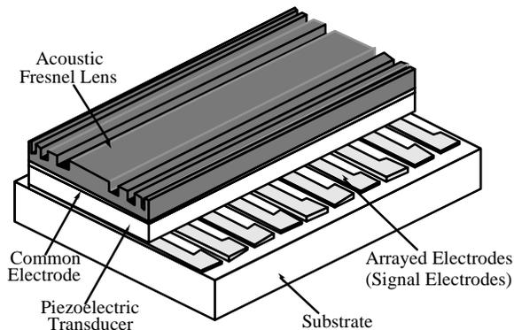
Figure 5. Structure of printing head with transducer arrays.
