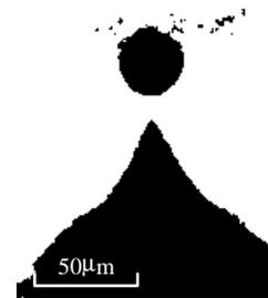
Figure 6. Photograph of droplet ejecting from free ink surface. The diameter of a droplet is approximately  $30\ \mu\text{m}$ .
