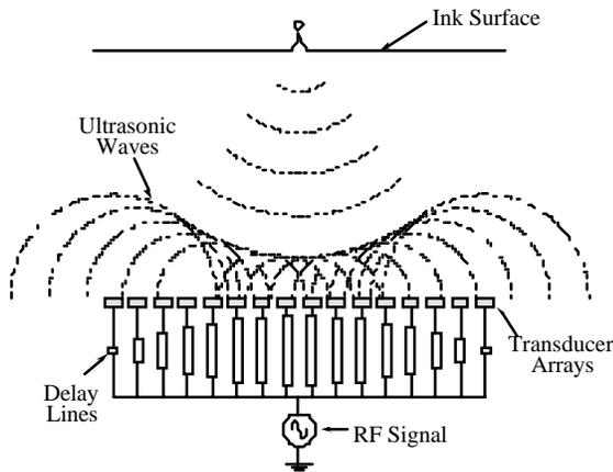
Figure 1. Schematic diagram of electronic focusing with transducer arrays.
