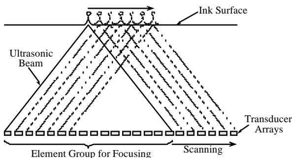
Figure 2. Schematic diagram of electronic scanning along transducer arrays.
