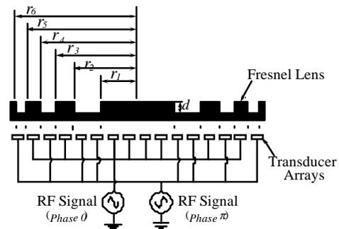
Figure 3. Schematic diagram of a cross-sectional Fresnel lens and assignment of RF signal phased arrays to transducer elements.
