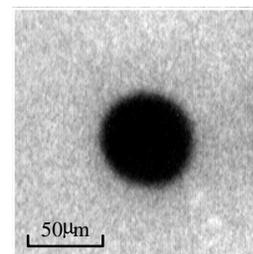
Figure 7. Photograph of a spot on silica-coated paper. The diameter of a spot is approximately  $60\ \mu\text{m}$ .
