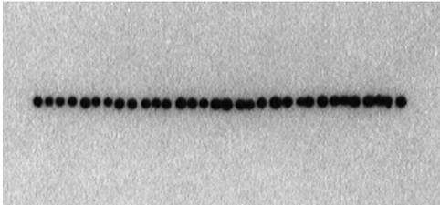
Figure 8. Spots on paper during electronic scanning of an ultrasonic beam consecutively.
