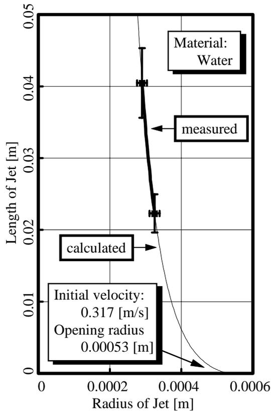
Figure 2: Thread-state jet form expressed by its length versus radius. Light line is theoretically calculated by (Eq.6). Heavy line is measured from Taylor's photographs by using microscope.
