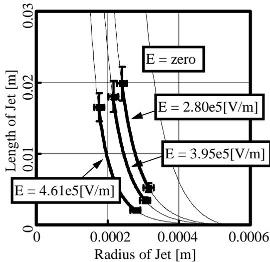
Figure 4: Electrically driven water jet transforming characteristics. Theoretically calculated light lines and experimentally measured heavy lines are plotted for the parameters of electrostatic field.
