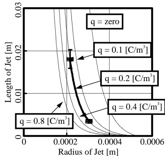
Figure 3: A group of jet forms calculated for several "q" parameters. The electrostatic field is constant at  $3.95 \times 10^5$  [V/m]. Experimentally measured heavy line shows a good agreement with 0.2 [ $C/m^3$ ] charged curve line.
