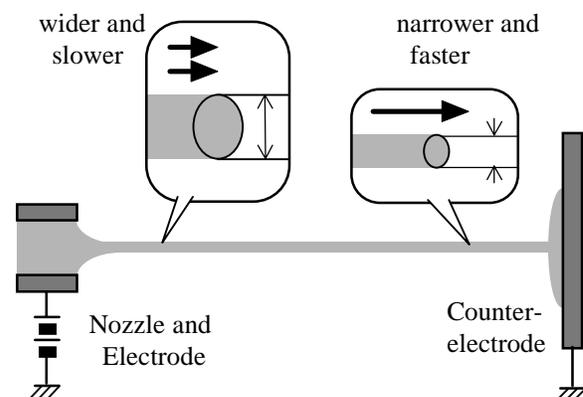
Figure 1: Simply illustrated thread-state liquid jet.
