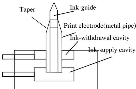
Figure 2. Cross-sectional view of the print head
