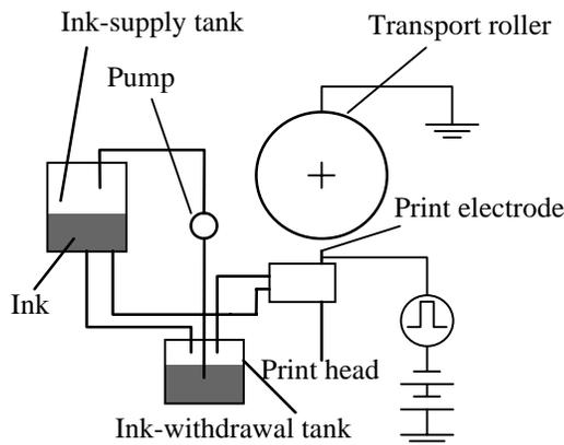
Figure 4. Schematic diagram of the experimental setup
