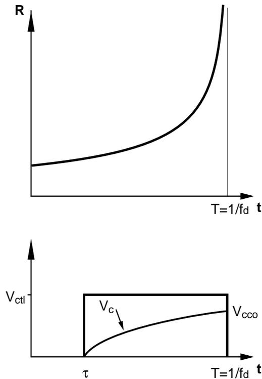
Figure 5. Principle for the applying of the region measurement pulse (RMP). The drop is charged during the on-time of the pulse.
