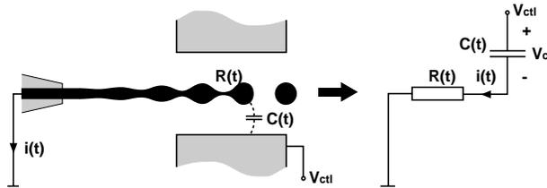
Figure 2. Electrical model of the charging of the drops
