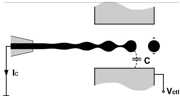
Figure 1. Electrical charging of a conducting continuous ink jet
