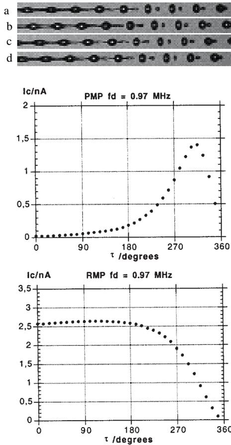
Figure 8. Results from the measurement of the width of the forbidden region for a drop formation frequency of 0.97 MHz. The satellite cut-off occurs after the main drop cut-off. The drop formation is shown above for a) 0, b) 90, c) 180 and d) 270 degrees phase with respect to the main drop cut-off.
