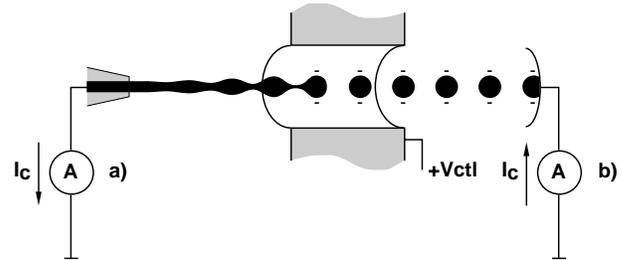
Figure 3. Charging current measurement. a) Through the ink ground terminal. b) Through discharging of the charged drop.
