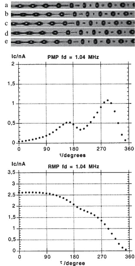
Figure 9. Results from the measurement of the width of the forbidden region for a drop formation frequency of 1.04 MHz. The satellite cut-off occurs before the main drop cut-off. The drop formation is shown above for a) 0, b) 90, c) 180, d) 225 and e) 270 degrees phase with respect to the main drop cut-off.
