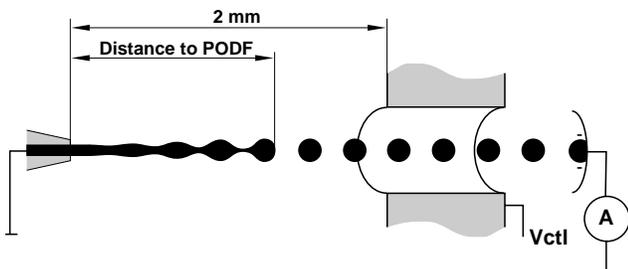
Figure 4. Experimental set-up for the measurement of the distance to the PODF.
