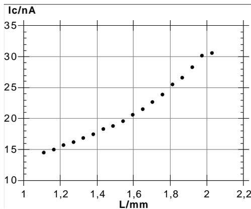
Figure 6. Charging current vs. the distance to the PODF for a 9.5 μm jet traveling at a velocity of 53 m/s. The stimulation frequency was set at 1.0 MHz and the charging voltage was 40 V.
