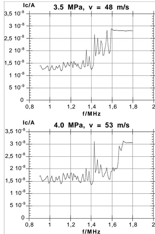
Figure 7. Charging current measured at two jet velocities when the stimulation frequency was varied between 0.9 - 1.8 MHz.
