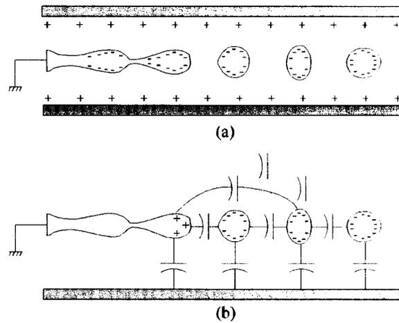
Figure 3. Charging geometry for a typical CIJ system.
