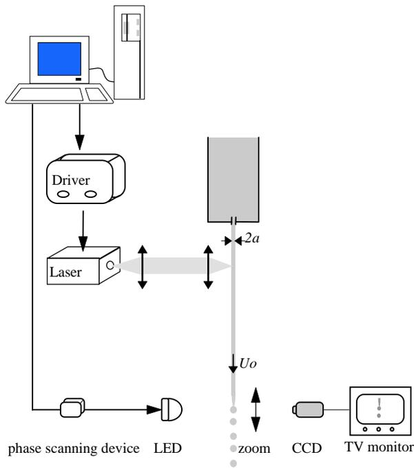
Figure 1 Schematic representation of the experimental set-up
