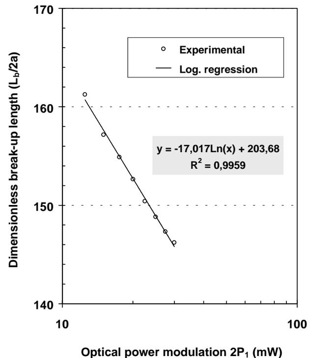
Figure 2 Jet break-up length as a function of the laser diode optical power,  $k = 0.71$ ,  $We = 102$ ,  $P_1 \in [10-30] \text{ mW}$
