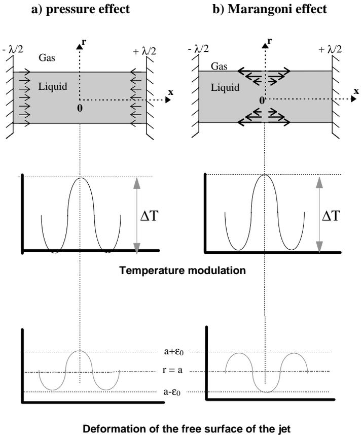
Figure 6 Schematic representation of the jet surface deformation induced by a pressure or Marangoni effect
