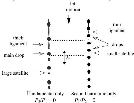
Figure 3 Typical jet break-up patterns
