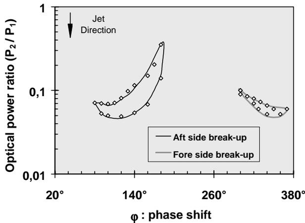
Figure 5 No-satellites areas at wave-number  $k = 0.43$  and jet velocity  $U_0 = 13.9$  m/s
