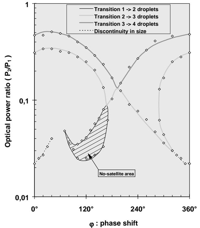
Figure 4 Jet break-up diagram at wave-number  $k = 0.40$  and jet velocity  $U_0 = 11.1$  m/s
