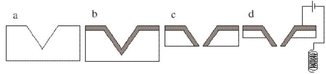
Figure 3 a: The flow channel and inverted pyramid is anisotropically etched. b: The backside of the wafer is n-doped (grey). c: The front side is anisotropically etched to attain the desired orifice size. d: The passivation voltage is turned on to protect the doped section and the pyramid shaped nozzle is uncovered when the etching is continued.
