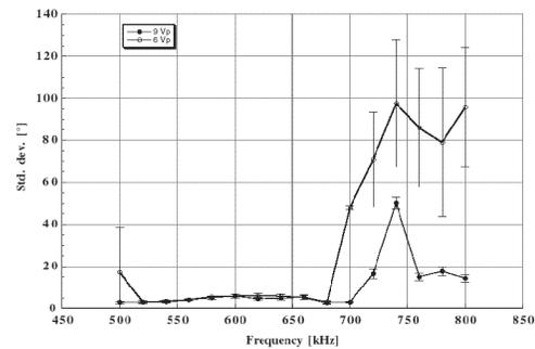
Figure 7. Standard deviation for time between droplets for a  $10 \times 10 \mu\text{m}$  nozzle measured at  $7 \text{ mm}$  from the orifice. The nozzle was operated at a flow of  $0.17 \text{ ml/min}$  which was achieved when a  $9.5 \text{ atm.}$  pressure was applied. The stimulation frequency was varied from  $500$  to  $800 \text{ kHz}$ .
