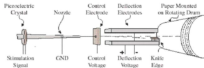
*Figure 1. The Hertz continuous ink jet printer principle. A control electrode, positioned at the point of droplet formation, charges the unwanted droplets and these are later deflected and caught by a knife edge. The uncharged droplets are not affected by the deflection field and hence hit the paper in the desired pixels.*
