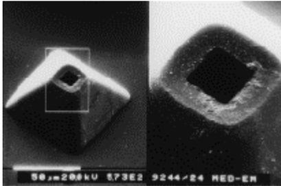
Figure 5. A top view of the nozzle captured with an SEM. The orifice size is approximately  $10 \times 10 \mu\text{m}$ . The small front area in combination with the pyramid-shaped nozzle reduces the risk of misalignment of the jet due to deposition of ink close to the orifice.
