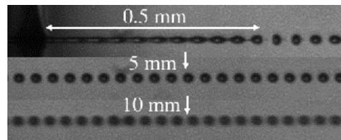
Figure 8. Images of droplets captured in stroboscopic light. At the point of droplet formation (top),  $5 \text{ mm}$  from the nozzle (middle) and at  $10 \text{ mm}$  from the nozzle. The stimulation frequency was  $590 \text{ kHz}$ .
