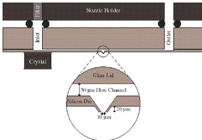
Figure 2. A cross-section of the nozzle structure. The dimensions for the flow channel in the nozzle prototype are (l) 13mm, (w) 2mm and (d) 30 $\mu\text{m}$ . The water-jet drilled holes in the glass lid have a diameter of 1 mm.
