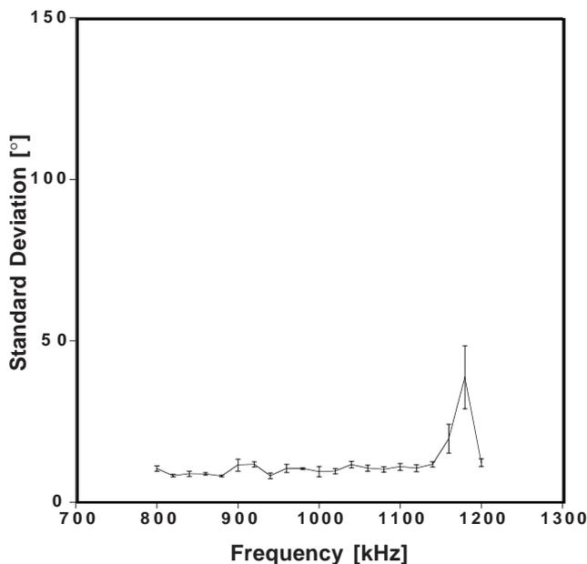
Figure 6. Measured droplet flight stability when the nozzle was stimulated at different frequencies. The measurements were conducted at 7 mm distance from the orifice of the nozzle. The amplitude of the stimulation signal is 10 Vpp.
