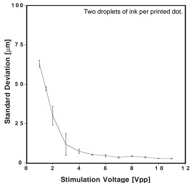
Figure 11. The standard deviation for distance between dots on paper. The dots contain two droplets of ink. The mean value for repeated measurements is represented by the line and the standard deviation for the measurements is presented as error bars.
