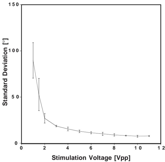
Figure 8. A plot of the influence of stimulation signal amplitude on the measured droplet flight stability measured at 7 mm distance from the nozzle. The standard deviation is decreasing rapidly for increased amplitudes when the voltage is below 4 Vpp. Five measurements were conducted at each voltage and the graph show the mean as well as the standard deviation as error bars. The frequency of the stimulation signal is 1 MHz.
