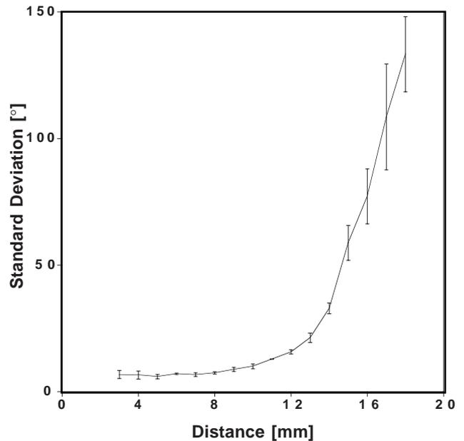
Figure 7. The measured droplet flight stability when the nozzle was stimulated with frequency of 1 MHz and the distance from the orifice of the nozzle to the point of measurement was varied. A non-linear change in measured standard deviation is detected when the distance from orifice is increased. The amplitude of the stimulation signal is 10 Vpp.
