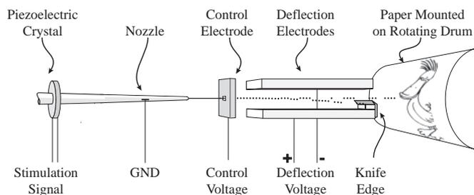
Figure 1. The Hertz continuous ink jet printer principle. A positive control voltage pulse with variable duration applied to the control electrode synchronized to the droplet formation process will cause charging of unwanted droplets. The charged droplets will be deflected downward and caught by the knife edge due to the high-voltage field between the deflection electrodes. The uncharged droplets will pass the deflection field unaffected and hit the paper in the desired pixel.
