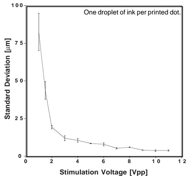
Figure 10. The standard deviation for distance between dots on paper. The dots contain one droplet of ink. The mean value for repeated measurements is represented by the line and the standard deviation for the measurements is presented as error bars.
