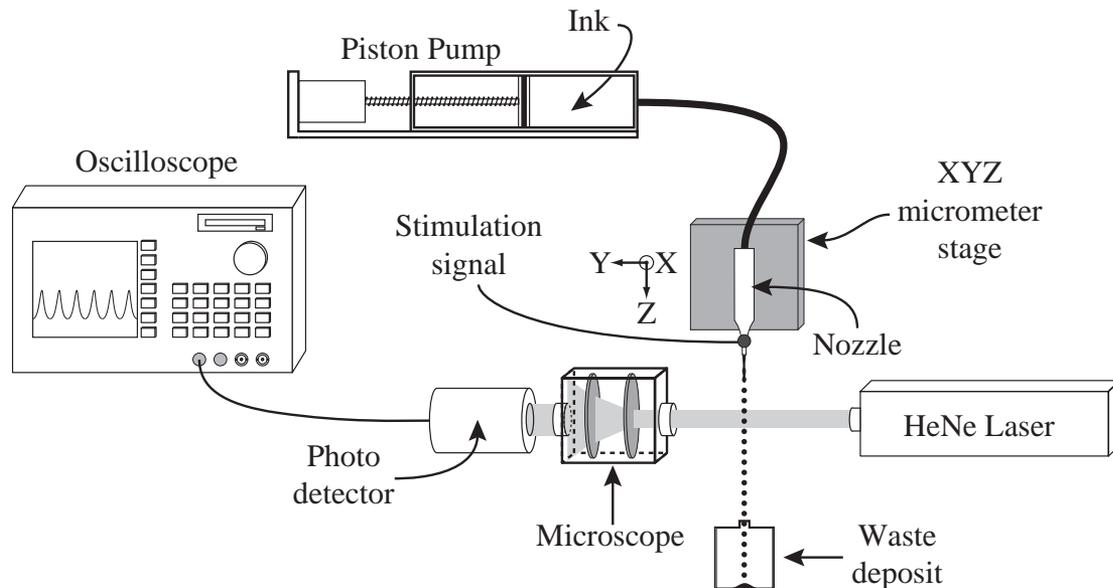
Figure 4. The optical droplet flight stability measurement setup.
