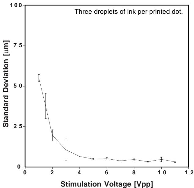
Figure 12. The standard deviation for distance between dots on paper. The dots contain three droplets of ink. The mean value for repeated measurements is represented by the line and the standard deviation for the measurements is presented as error bars.
