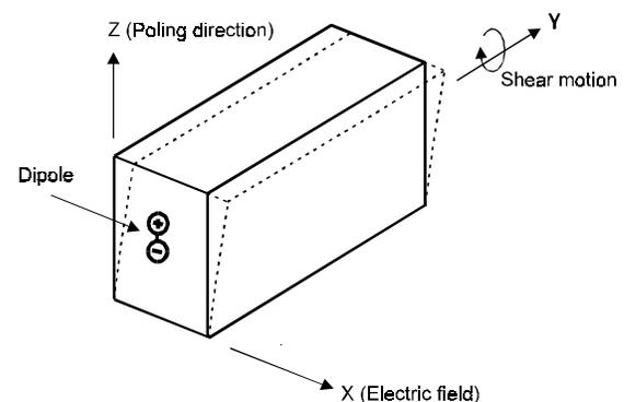
Figure 2. Shear mode actuation of PZT by an external electric field
