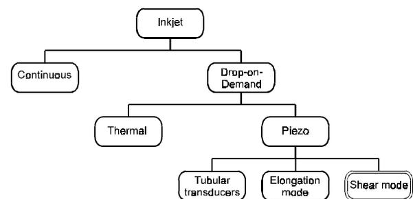
Figure 1. Inkjet actuator construction principles
