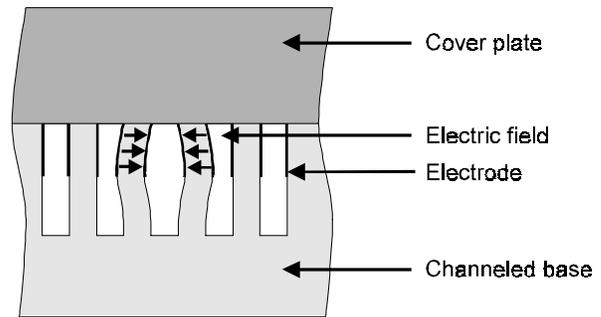
Figure 5. Usage of electric fields and shear motion for drop generation
