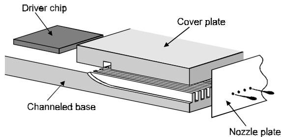
Figure 3. Basic printhead components
