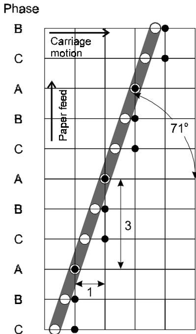
Figure 6. Tilting the printhead for a given resolution
