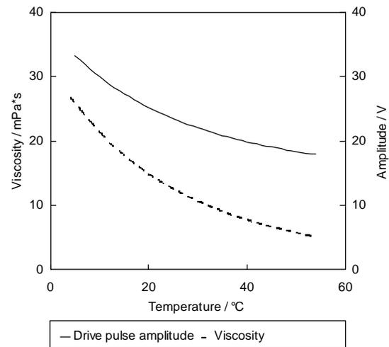
Figure 10. Ink viscosity (dashed curve) and drive pulse amplitude (solid curve) as a function of the temperature
