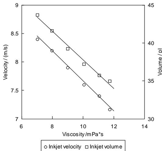
Figure 9. Inkjet velocity and volume as a function of the ink viscosity
