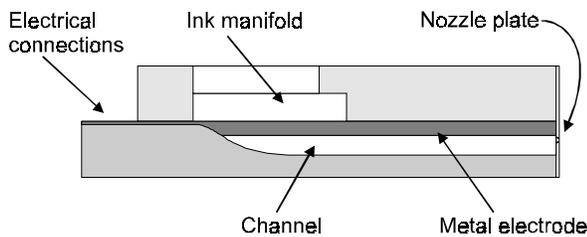
Figure 4. Cross-section of the actuator parallel to the channels
