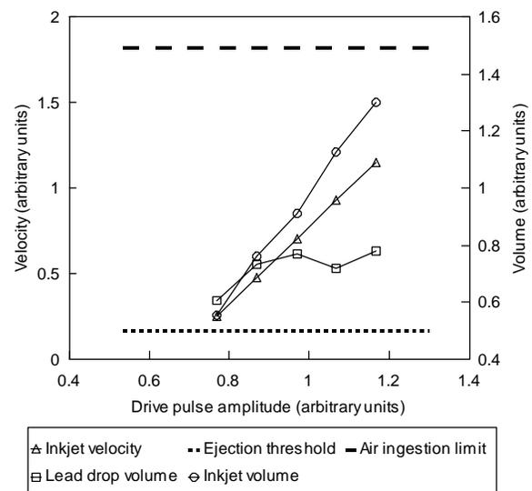
Figure 8. Inkjet volume, lead drop volume and velocity as a function of the drive pulse amplitude
