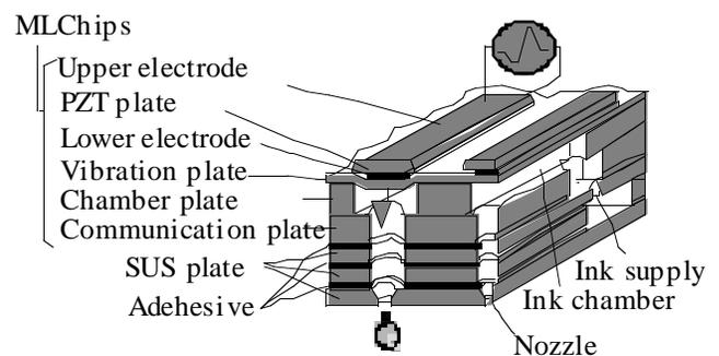
Figure 1: The composition of MLChips type head
