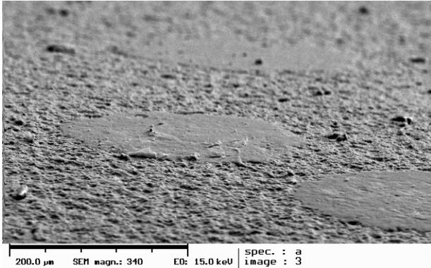
Figure 2. Hot-melt dot on an Aluminium surface
