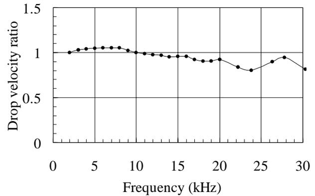
Figure 3. Drive frequency vs. Drop velocity ratio . Drop velocity ratio is given by measurement value divided by 13m/s. Drive voltage is constant at 2kHz.
