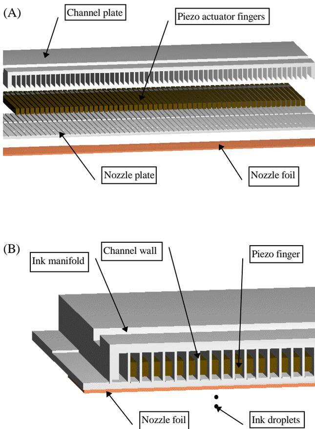
Figure 2: Major parts of a bend mode actuator printhead (A) before assembly (B) assembled
