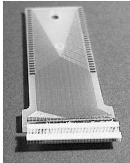
Figure 8: Prototype of a bend mode actuator printhead
