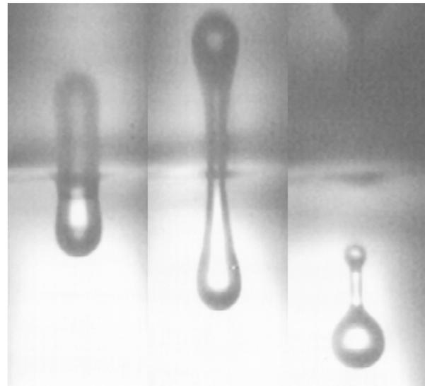
Figure 7: Droplet ejection of a bend mode printhead
