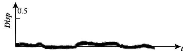
Figure 7. Normalized PZT displacement four chambers away from the active pressure chamber.
