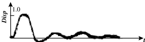
Figure 5. Normalized PZT displacement at an active chamber.
