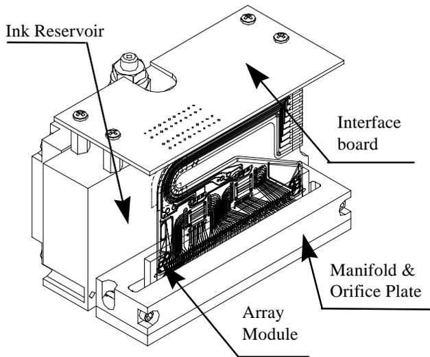
Figure 1. Spectra's 128 jets, 600dpi CCP Printhead.
