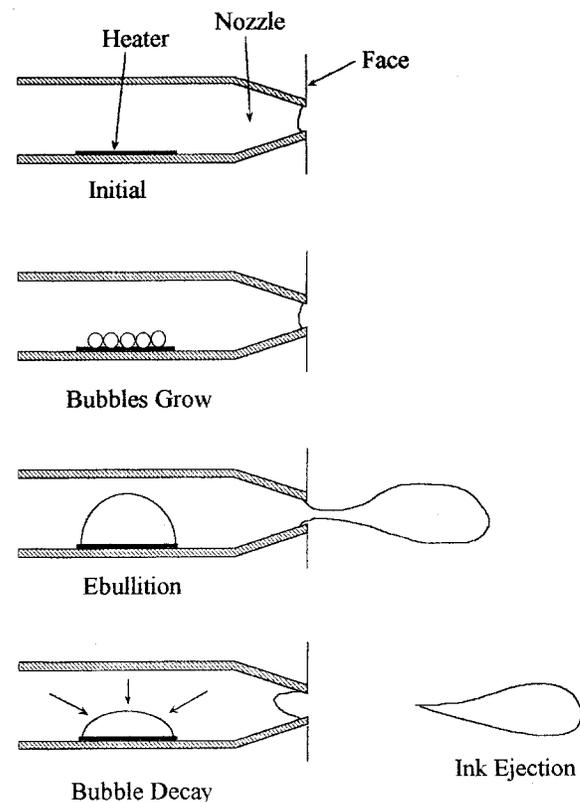
Figure 1. Ink Ejection of Bubble-jet printer
