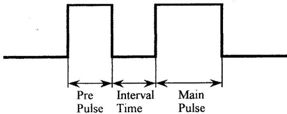
Figure 2. Double Pulse Wave Form
