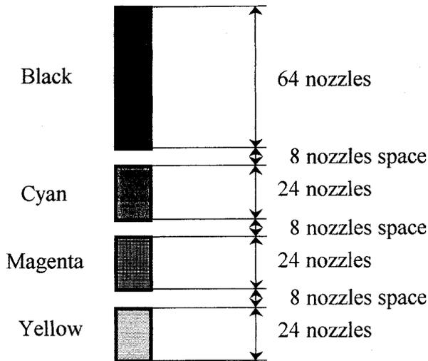
Figure 4. BC21 (Color Head for BJC-4000) Nozzle Layout
