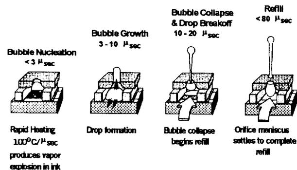
Illustration 4: Vaporization Principle of Drop Ejection: No moving parts except the ink itself
