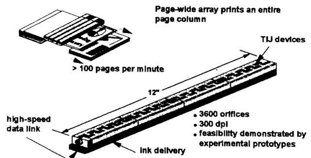
Illustration 15: Page Wide Arrays. High Throughput from a Large Array of Orifices.
