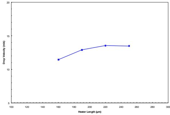
Figure 1: Drop velocity as a function of heater length at 32 °C
