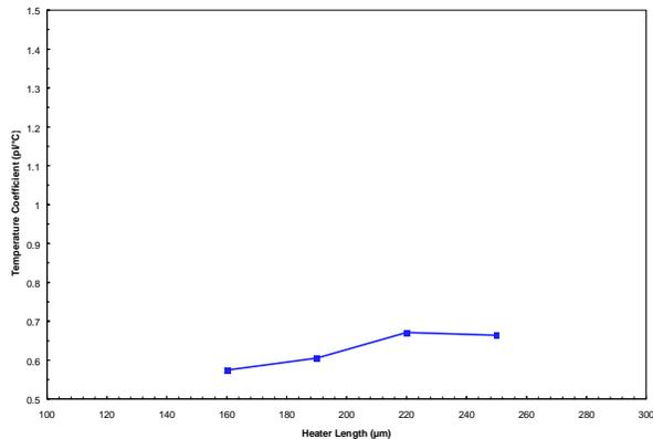
Figure 7: Drop volume temperature coefficient as a function of heater length
