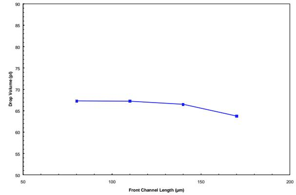
Figure 4: Drop volume as a function of front channel length at 32 °C
