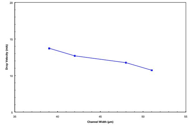
Figure 5: Drop velocity as a function of channel width at 32 °C
