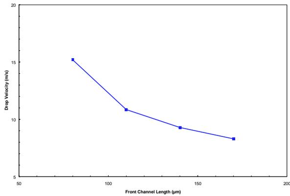
Figure 3: Drop velocity as a function of front channel length at 32 °C
