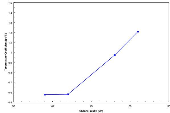
Figure 9: Drop volume temperature coefficient as a function of channel width
