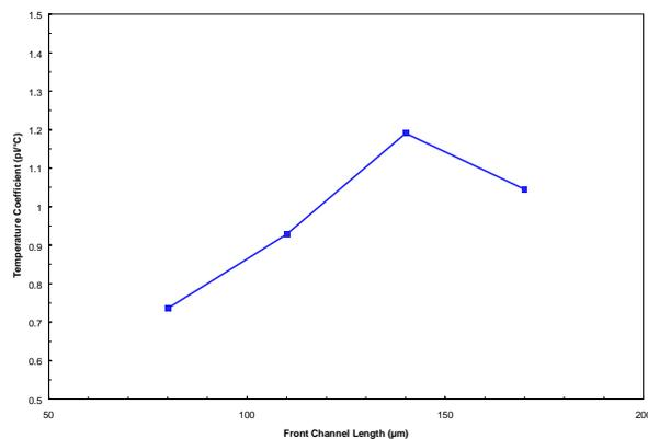
Figure 8: Drop volume temperature coefficient as a function of front channel length
