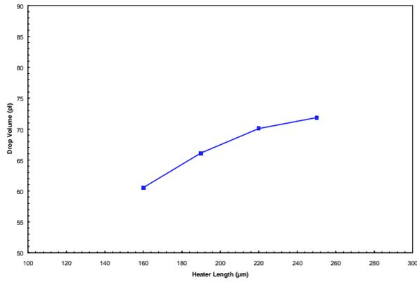
Figure 2: Drop volume as a function of heater length at 32 °C
