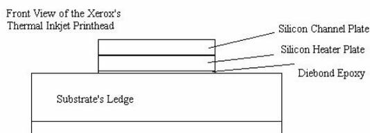
Figure 3. Front View of just the chip and substrate of Xerox's Thermal Inkjet Printhead
