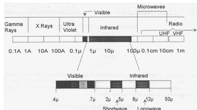
Fig. 1 Electromagnetic Spectrum Ref. [1]
