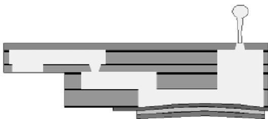
Figure 2. Cross-section of piezoelectric firing chamber
