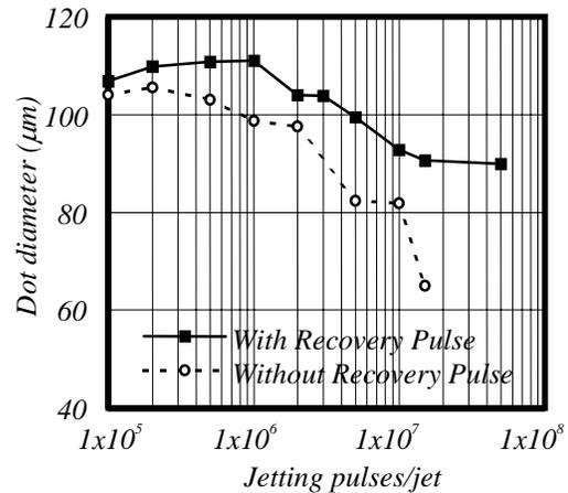
Figure 10. Dot diameter degradation by kogation
