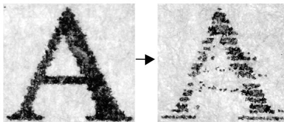
Figure 3. Print quality degradation by kogation.
