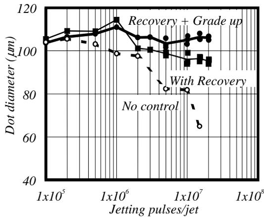
Figure 11. Dot diameter variation by optimized drive pulse.
