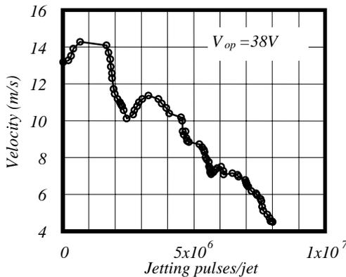
Figure 5. Change in drop velocity as a function of pulse number.
