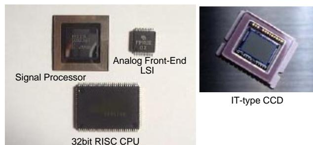
Figure 1. LSIs for this camera system
