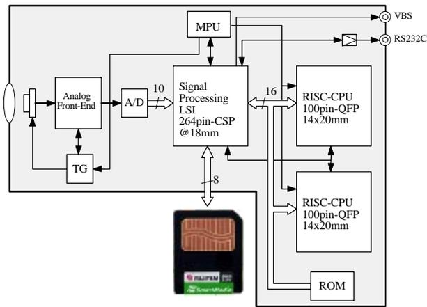
Figure 2. A Block Diagram for MX-600 ZOOM
