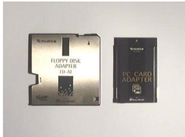
Figure 5. PC Interface (FD-A1/PC-AD3)
