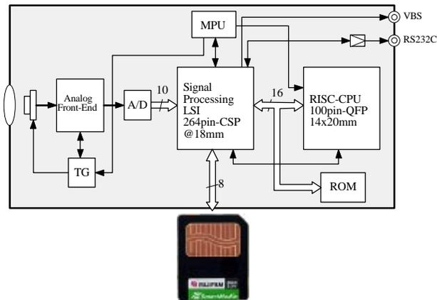
Figure 3. A Block Diagram For MX-500
