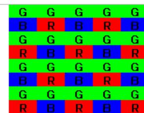
Figure 2. An example of color filter arrangement for dual pixel sensor
