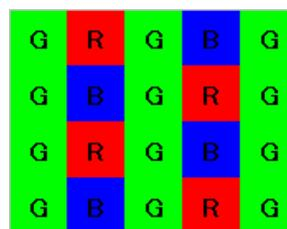
Figure 1. An example of color filter arrangement for conventional sensor
