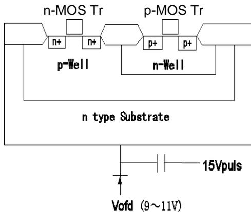
Figure 8. Cross section of CMOS
