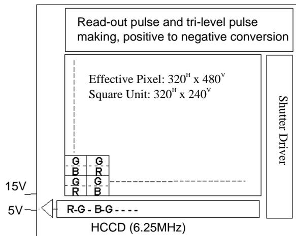
Figure 7. Block Diagram of Dual Pixel CCD
