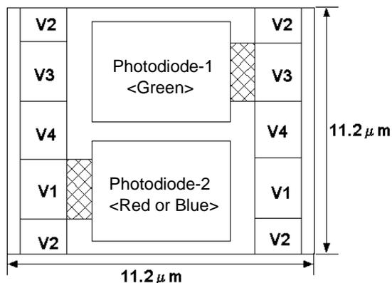
Figure 6. Pixel Layout of Dual Pixel CCD
