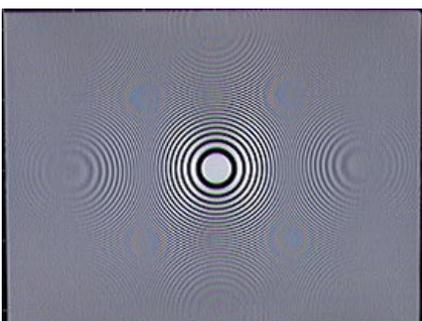
Figure 4. QVGA Image of CZP chart by Dual Pixel Sensor
