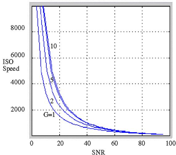
Figure 6. CMOS image sensor ISO speed vs. SNR
