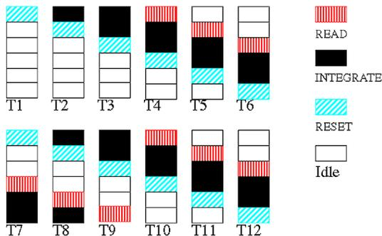
Figure 5. Rolling electronic shutter reset and readout progression
