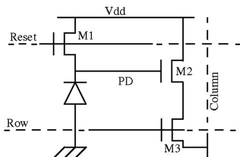
Figure 2. Pixel schematic
