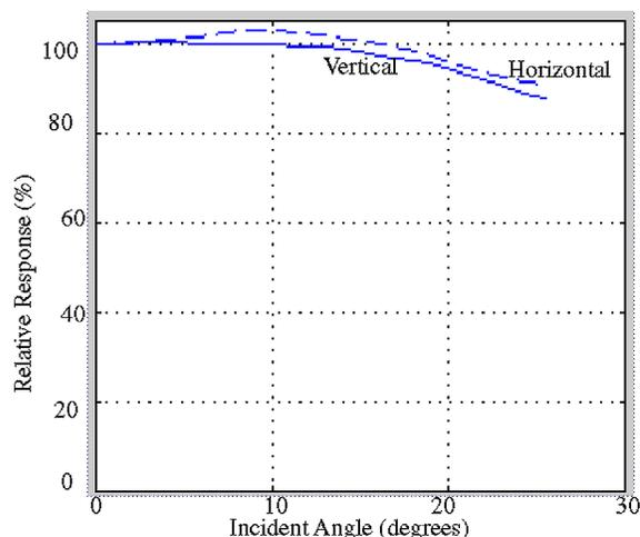
Figure 4. Pixel angular response
