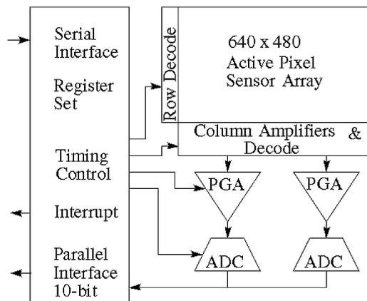
Figure 1. Imager block diagram
