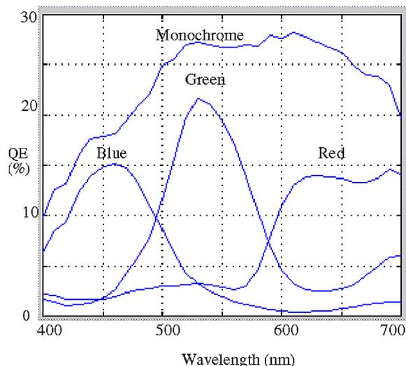
Figure 3. Pixel quantum efficiency without micro lens
