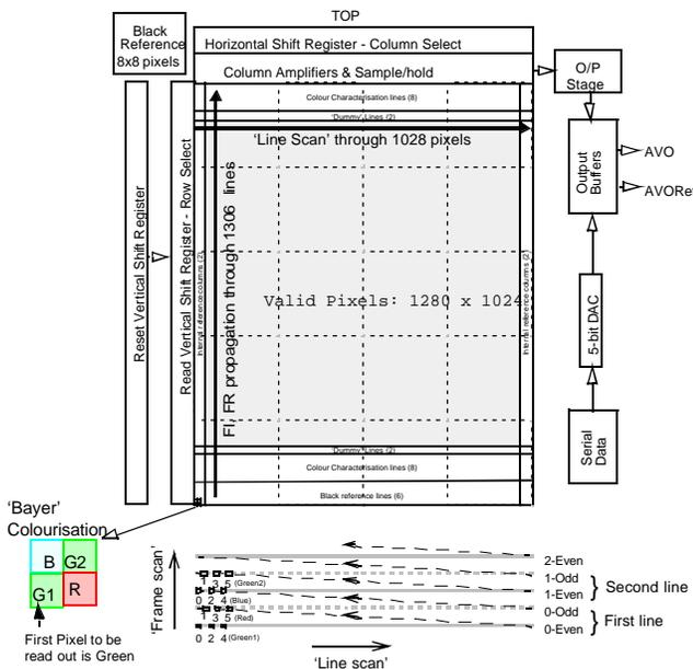
Figure 1.0 Sensor Array Architecture
