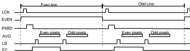
Figure 1.2 Line Readout Timing
