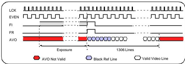
Figure 1.1 Single Frame Integration & Readout
