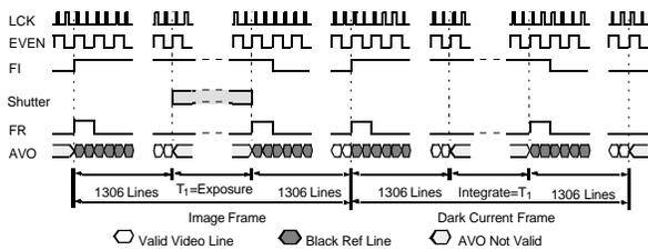
Figure 3 : Relative timing of still image capture with frame buffer
