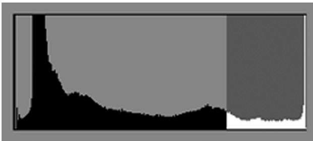
Figure 4. Overexposure with Capture Mean of 213 ADU
