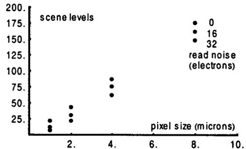
Figure 4. Scene-levels as function of pixel size and read-noise
