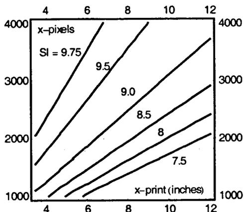
Figure 6. Sharpness as function of print-size and pixel-number.
