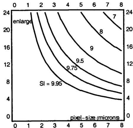
Figure 5. Sharpness as function of pixel-size and enlargement .
