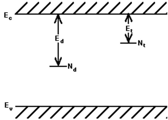
Figure 1. Energy structure of AgX with traps  $N_t$  and intrinsic defect levels  $N_d$ .
