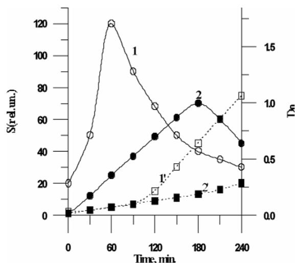
Figure 3. The kinetic of chemical sensitization of emulsion with epitaxial tabular microcrystals AgBr/AgCl (1, 1') and without epitaxes (2, 2').
