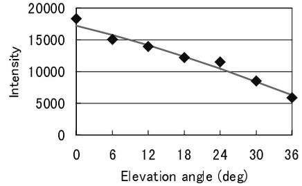
Figure 2. Intensity of diffuse component vs. illumination angle.
