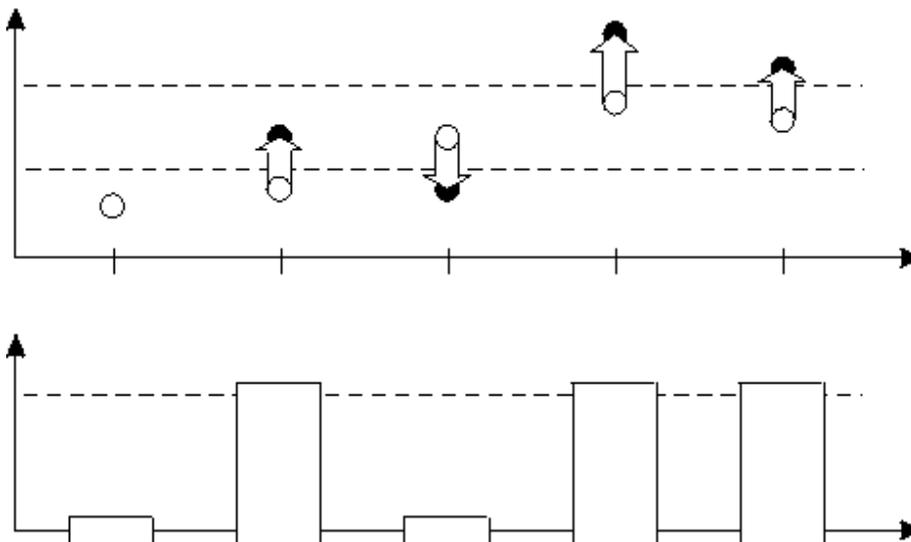
Figure 1. The continuous tone input data (gray circles top) is quantized to the binary output (gray rectangles bottom) generating a quantization error (white arrows). This error is used to create a modified input (black circles top) for subsequent pixels.
