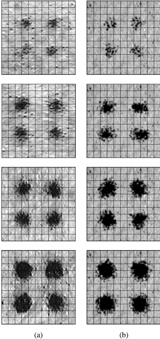
Figure 2: Dot clusters composed of one, two, three or four black pixels for (a) an Apple LaserWriter Pro 630 printer and (b) a stochastic dot model.
