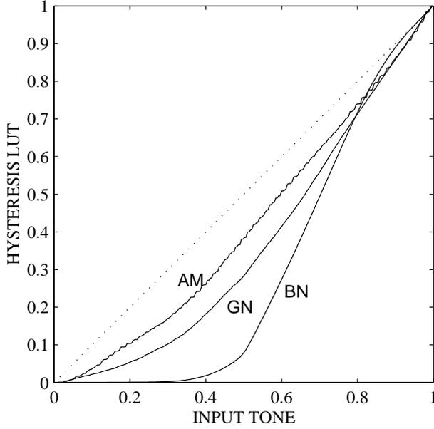
Figure 4: Modeled tone reproduction curve using clustered-dot ordered dither ( $8 \times 8$  cells), blue-noise, and green-noise halftoning.
