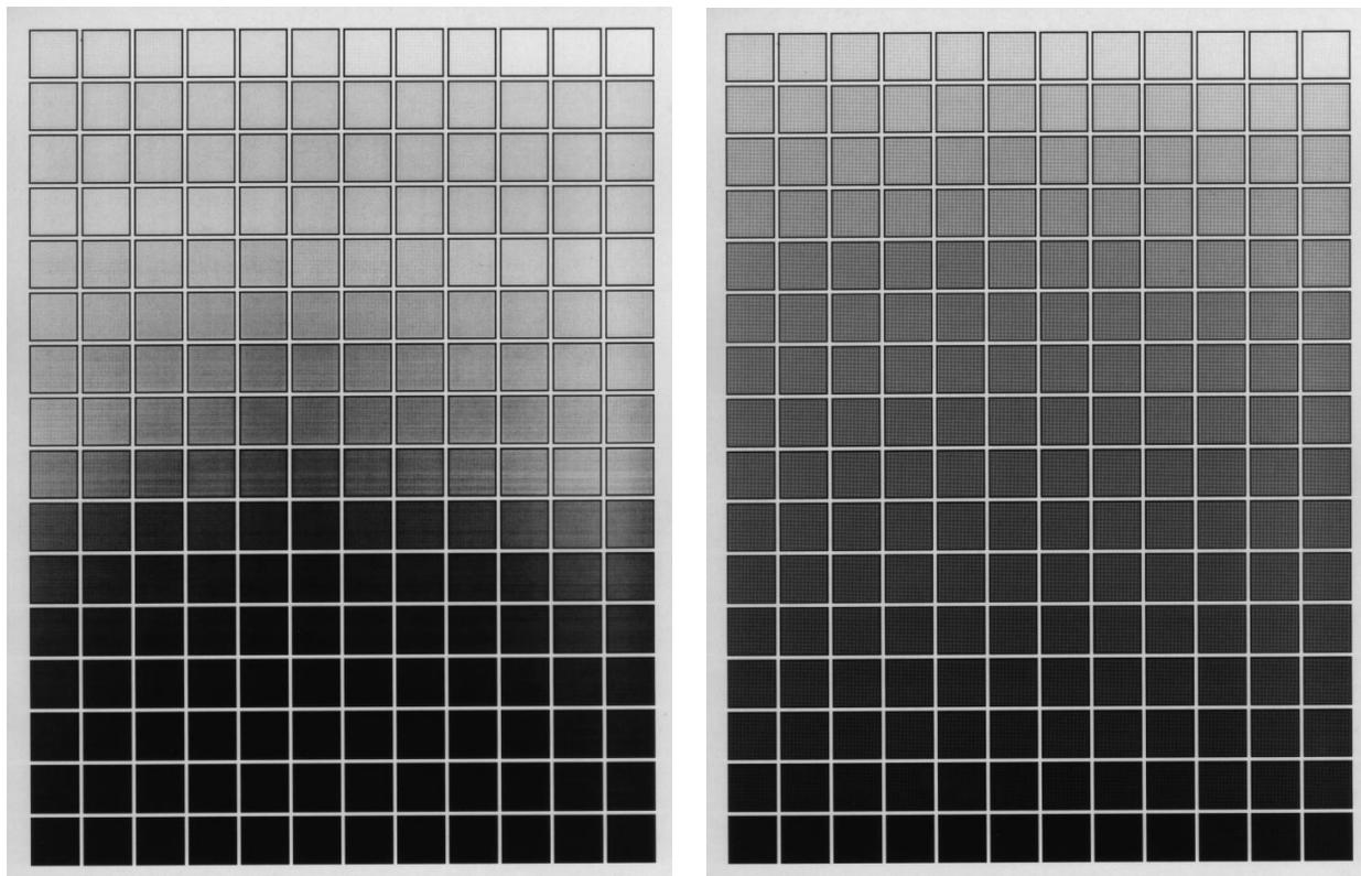
Figure 1: Gray-scale ramps printed on an Apple LaserWriter Pro 630 using (left) Bayer's dither, illustrating dot-loss, and (right) CDOD with  $8 \times 8$  cells.
