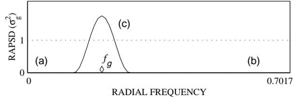
Figure 3: The radially averaged power spectrum density for the ideal green-noise halftone pattern.
