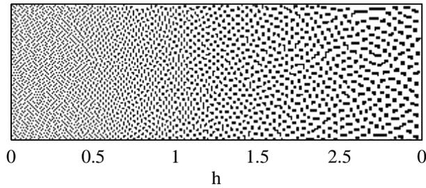
Figure 7: Halftoned image ( $g = 0.75$ ) showing the effects of increasing  $h$ .
