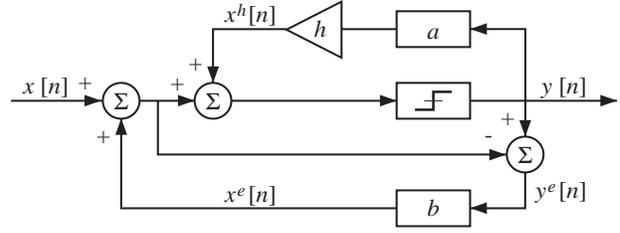
Figure 5: The error diffusion with output-dependent feedback algorithm as introduced by Levien [6].
