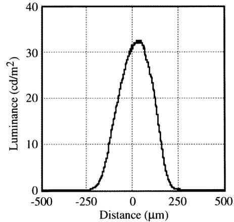
Figure 2. The measured LSF of the CRT monitor used in the experiment.
