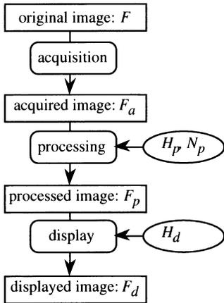
Figure 3. Imaging system for preparing the samples. Response function and noise level in the image processing device are changed in 6 levels each.
