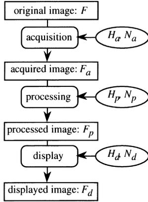
Figure 1. Schematic diagram of digital imaging system consisting of image acquisition, processing, and display device.
