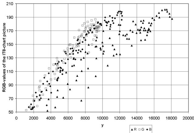
Figure 8. Evaluation of the spectral response showing the RGB data in relation to the calculated data; Camera: Canon PowerShot A5
