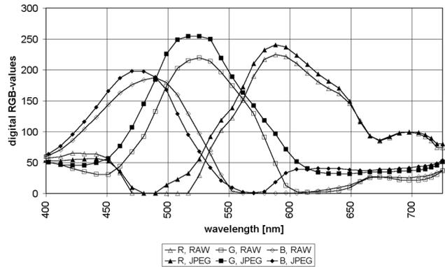
Figure 7. Comparison of RGB-values using different file formats; Camera: Canon PowerShot A5
