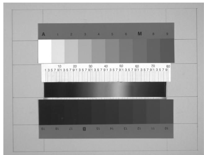
Figure 2. test chart with continuous Interference Filter
