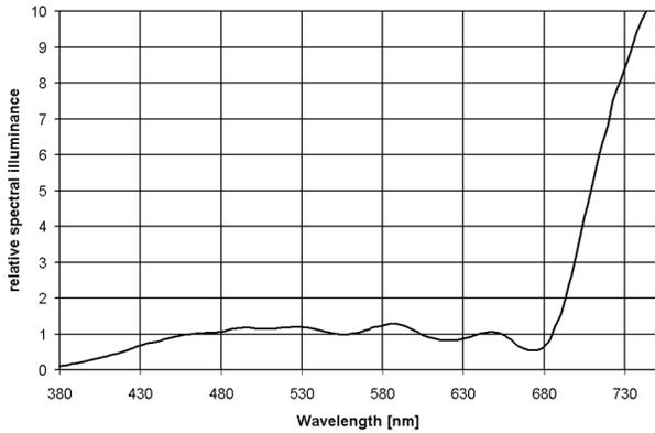
Figure 3. relative spectral illuminance of the interference filter.
